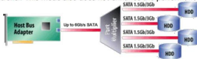
SATA PM connectivity: one port, one cable, four drives; 4-ports = 16 drives
